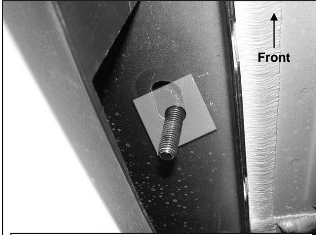
(Fig 5) Thread Plastic Retainer onto Bolt Plate
