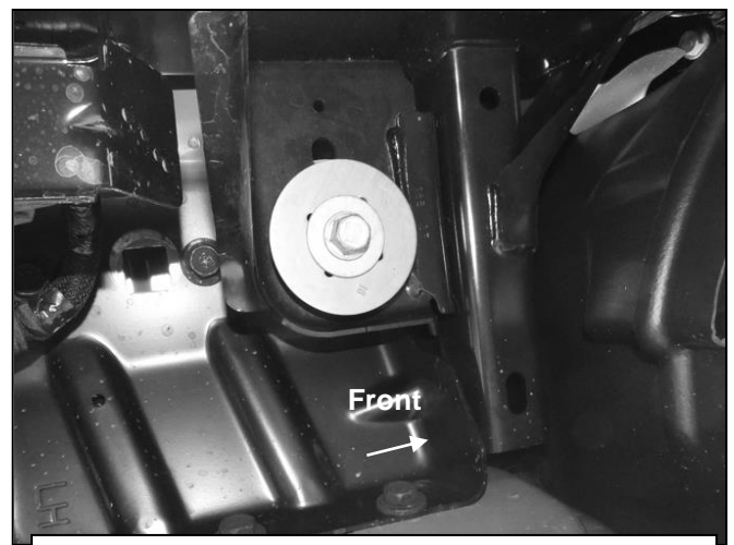
(Fig 4) Locate driver/left side front body mount
