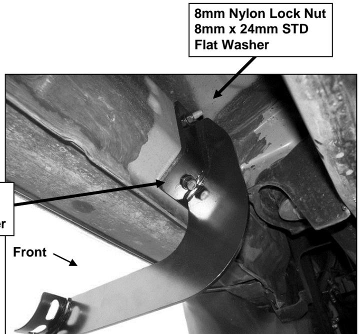
(Fig 2) Driver side front mounting location pictured
