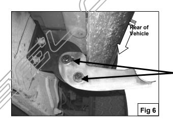
10mm x 30mm Hex Bolts 10mm Lock Washers 10mm Flat Washers Or **Factory Bolts**
