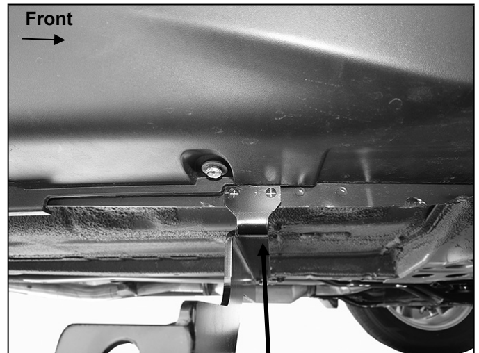
(Fig 14) Passenger front Bracket location marked before drilling
