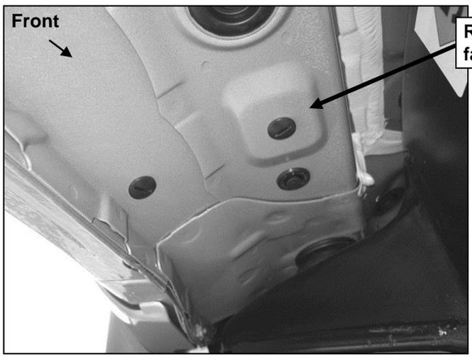
(Fig 1) Driver side front mounting location pictured
