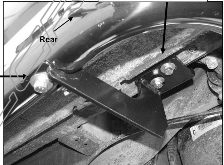
(Fig 4) Driver Side Center Mounting Bracket Pictured
