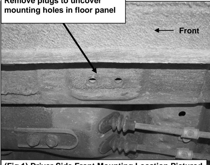
(Fig 1) Driver Side Front Mounting Location Pictured
