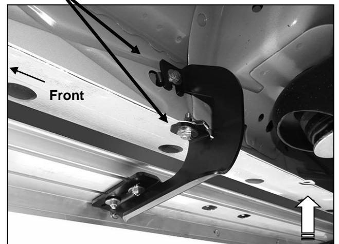
(Fig 13) Passenger/right center pictured. NOTE: On some models, center Bracket may not clear center body mount. Use either the mounting location in front of or behind the center body mount as necessary for Bracket clearance, (also see Figure 1 for additional info)
