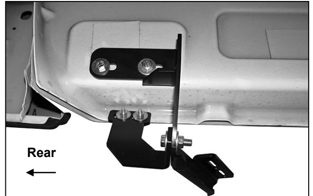
(Fig 17) Driver/Left rear Brackets installed (Example of Quad and Crew Cab)
