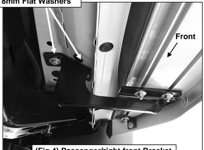
(Fig 4) Passenger/right front Bracket pictured with Running Board
