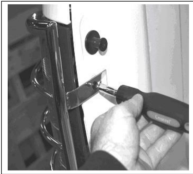
FIG. 3 Stock taillight mounting screws reinstall through inside brackets.
