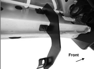
(Fig 6) Driver side front Bracket installed
