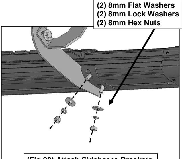
(Fig 20) Attach Sidebar to Brackets
