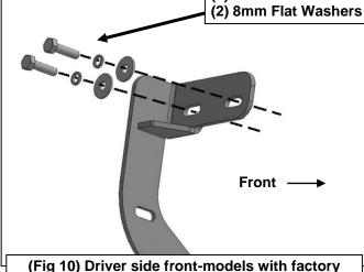
installed threaded inserts. Bolt Plate not required
