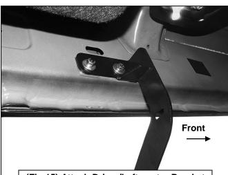
(Fig 15) Attach Driver/Left center Bracket
