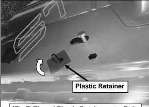
(Fig 5) Thread Plastic Retainer onto Bolt Plate to hold Bole Plate in position.
