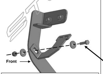
8mm Hex Bolt (2) 8mm Flat Washers 8mm Nylon Lock Nut
