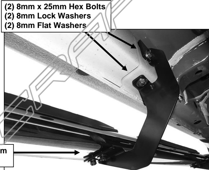
(Fig 6) Passenger side center Bracket installation
