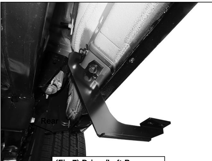
(Fig 7) Driver/Left Rear Mounting Bracket installed
