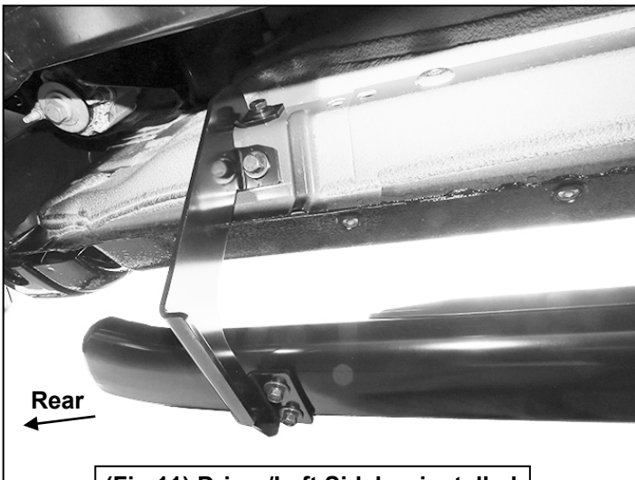
(Fig 11) Driver/Left Sidebar installed on Rear Mounting Bracket
