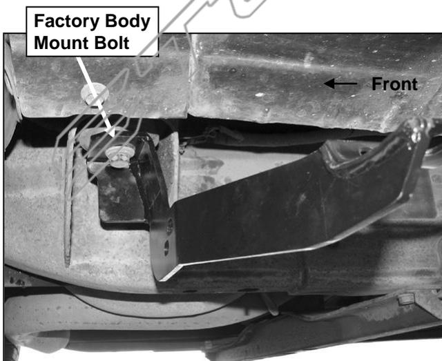
**(Fig 1) Driver side front mounting bracket pictured**
