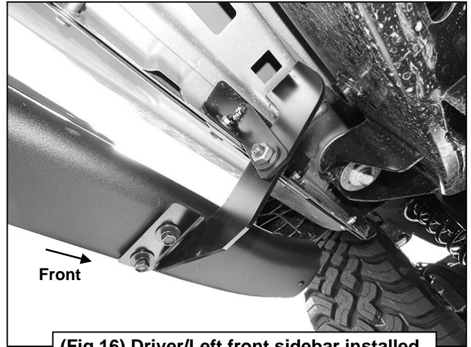
(Fig 16) Driver/Left front sidebar installed
