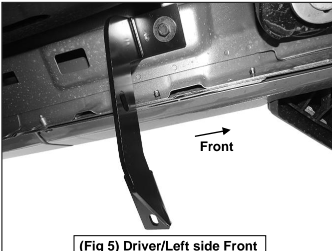
(Fig 5) Driver/Left side Front Mounting Bracket attached
