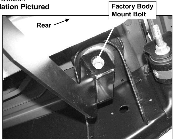
**(Fig 2) Driver side rear mounting bracket pictured**
