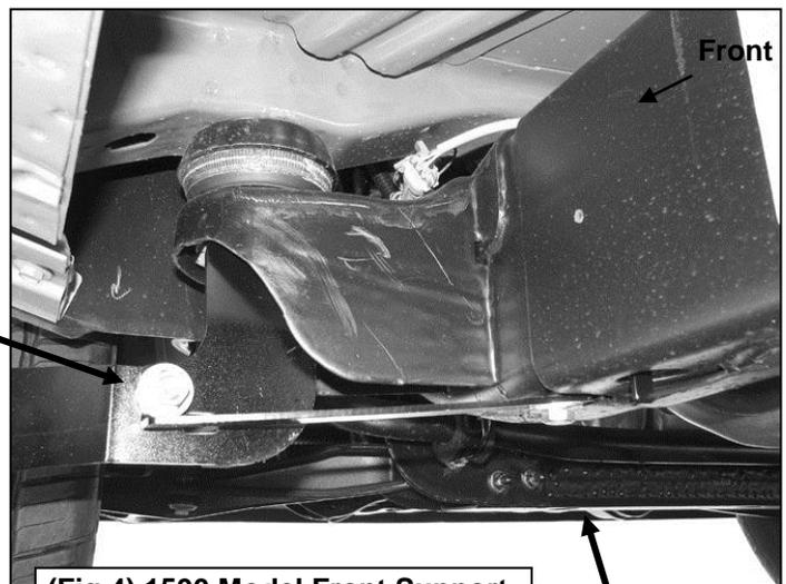
(Fig 4) 1500 Model Front Support Bracket Installation Pictured
