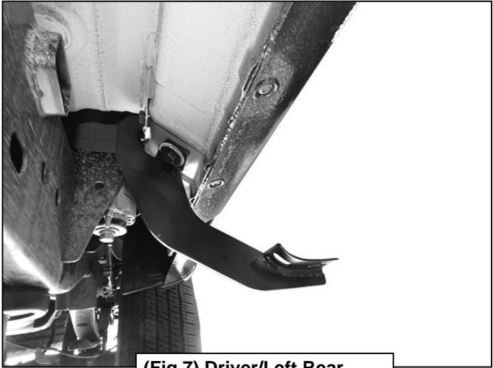
(Fig 7) Driver/Left Rear Mounting Bracket installed
