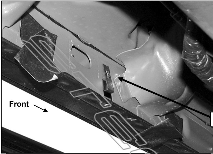
(Fig 4) Driver side-center Mounting Bracket location
