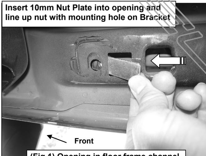
Insert 10mm Nut Plate into opening and line up nut with mounting hole on Bracket
