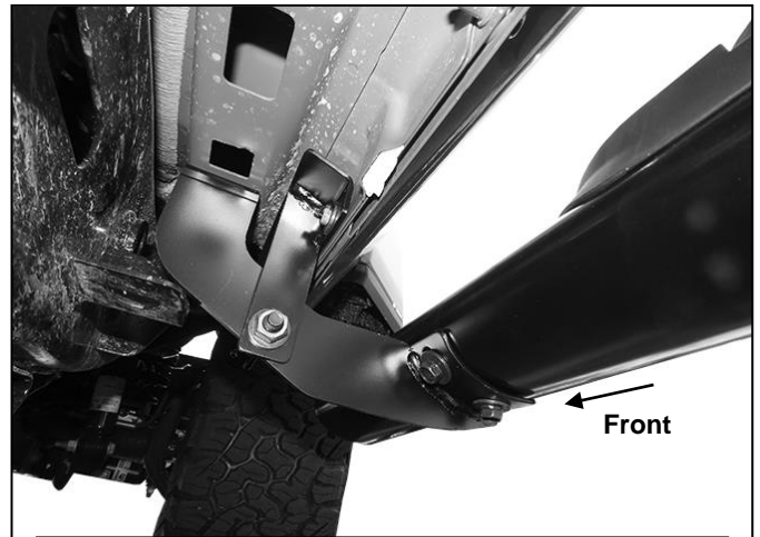
(Fig 16) Passenger/Right front sidebar installed
