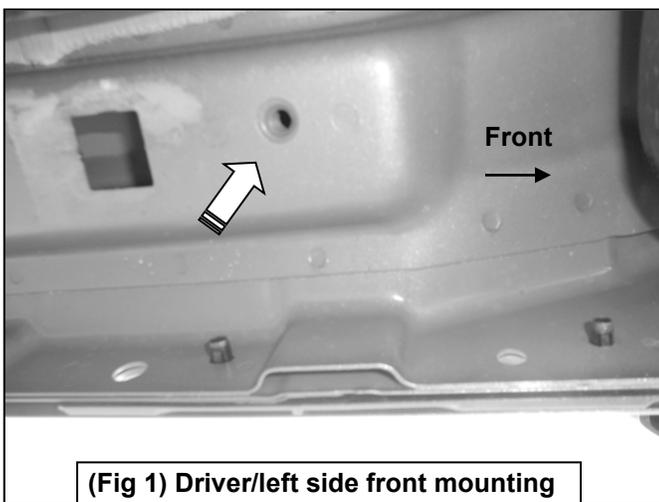
(Fig 1) Driver/left side front mounting location with threaded insert
