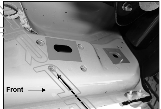
(Fig 9) Driver side front mid 2015-on, an example of models with factory installed threaded inserts
