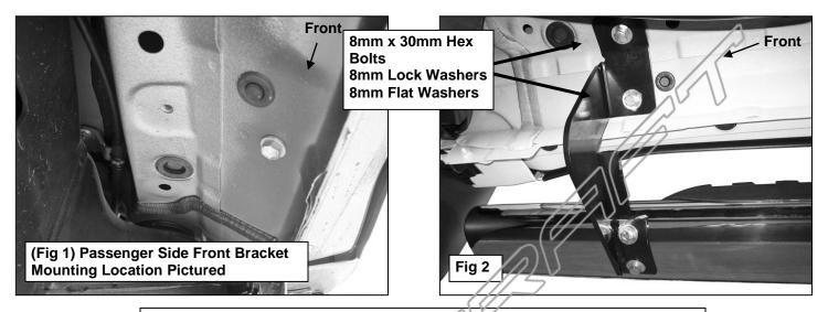
There are four sets of threaded holes in the side panel. Starting from the front of the vehicle, use the first, second, and fourth set of holes.
