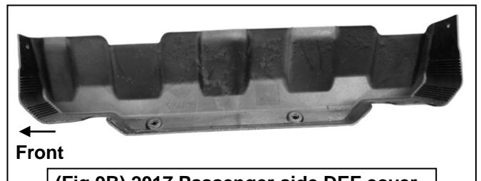
(Fig 9B) 2017 Passenger side DEF cover
