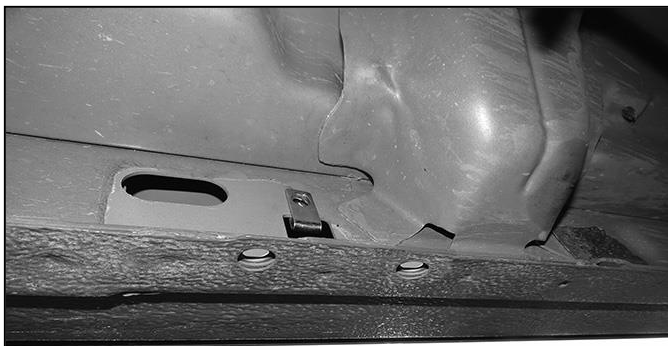
(Fig 4) Driver/left side Front Bracket attached to pinch weld illustrated
