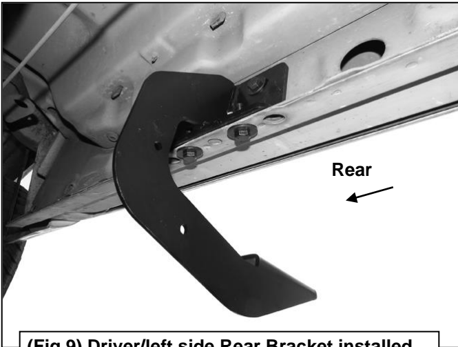
(Fig 9) Driver/left side Rear Bracket installed
