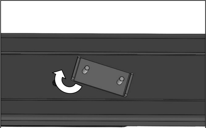
(Fig 9) Insert 8mm Double Bolt Plate through the channel opening in the bottom of the Sidebar
