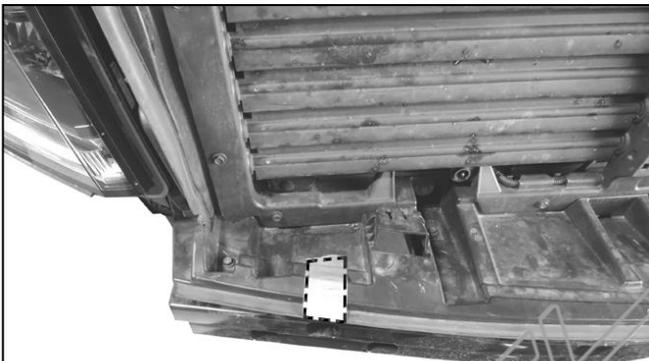
**(Fig 7) Passenger side approximate cut out on Plastic cover to clear Bracket**
