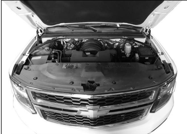
**(Fig 1) Remove plastic cover from top of grille**
