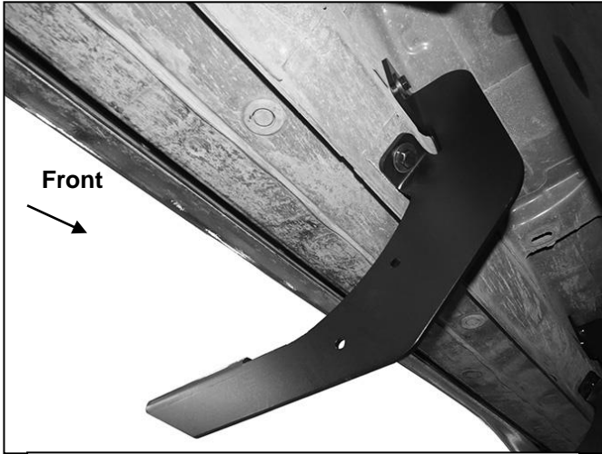
(Fig 4) Driver/left center Bracket installed Note: all cradles face towards front of vehicle
