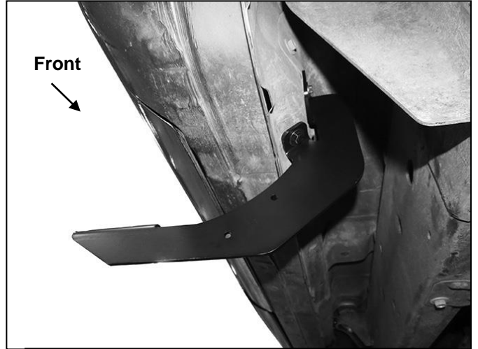
(Fig 5) Driver/left rear Bracket installed Note: all cradles face towards front of vehicle
