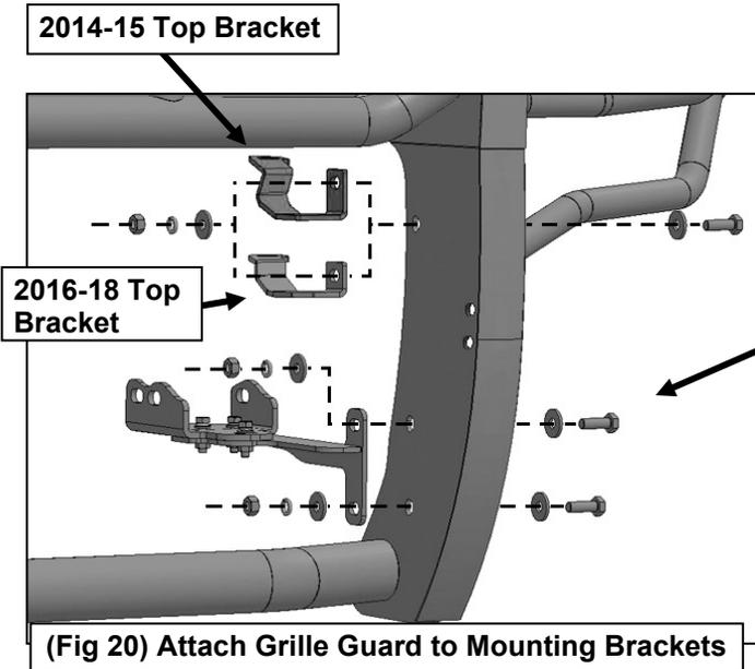
**(Fig 20) Attach Grille Guard to Mounting Brackets**
