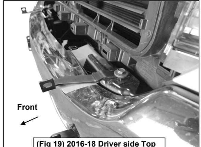
**(Fig 19) 2016-18 Driver side Top Mounting Bracket installed**
