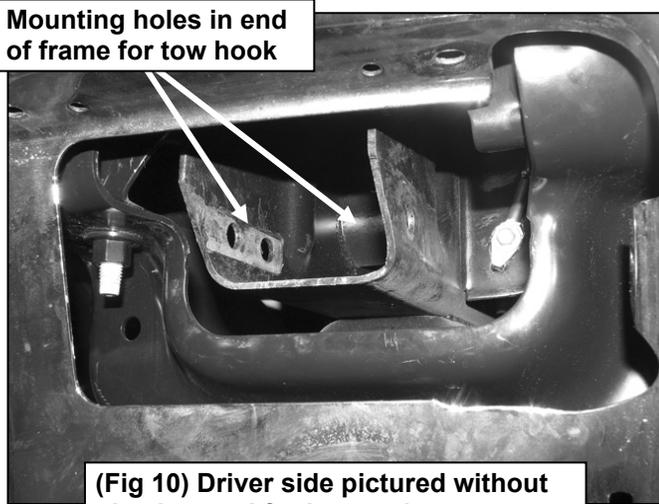
**Mounting holes in end of frame for tow hook**
