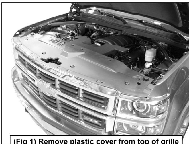
**(Fig 1) Remove plastic cover from top of grille**
