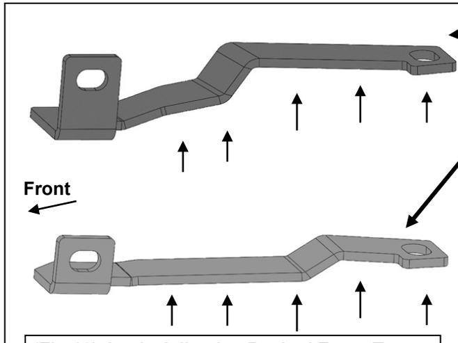
**(Fig 18) Apply Adhesive Backed Foam Tape to the underside of Top Mounting Bracket**
