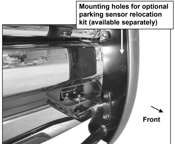
**(Fig 21) Attach Grille Guard to Mounting Brackets**
