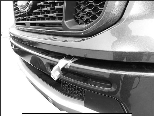
(Fig 12) Support Brackets attached
