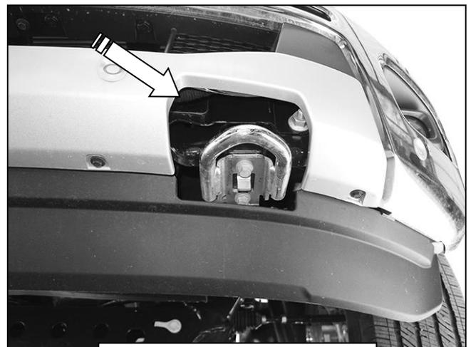
**(Fig 2) Remove plastic cover surrounding tow hook**
