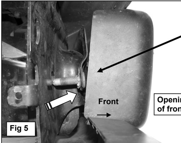
Hold the bumper bolt out of the way and insert Frame Bracket between bumper cover and bumper bracket. Line up hole in Bracket with bumper bracket and reinsert bumper bolt
