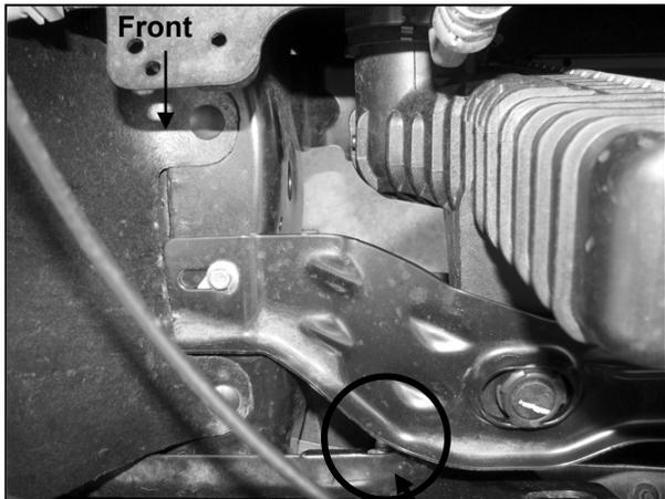
(Fig 2B) Remove bumper bracket hex nuts
