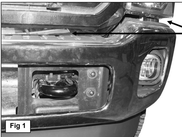
Before removing bumper bolts, measure gaps above bumper on driver and passenger side to relocate bumper
