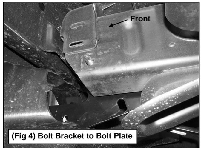
(Fig 4) Bolt Bracket to Bolt Plate
