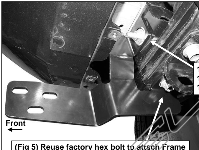
(Fig 5) Reuse factory hex bolt to attach Frame Bracket to bottom of cross-member
