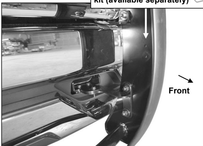
(Fig 21) Attach Grille Guard to Mounting Brackets
