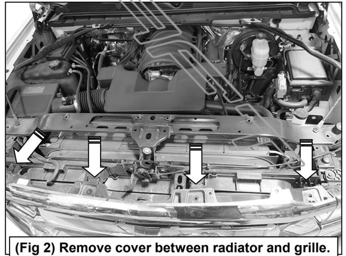
**(Fig 2)** Remove cover between radiator and grille. Remove screws attaching top of grille (arrows)
