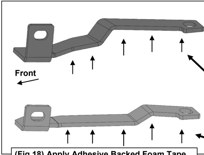
**(Fig 18) Apply Adhesive Backed Foam Tape to the underside of Top Mounting Bracket**
