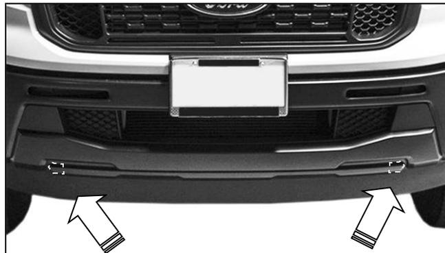
(Fig 5) Models without tow hooks, cut openings in lower plastic cover to clear Brackets
