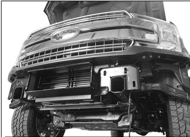
(Fig 18) 2018 models: Remove bumper assembly
