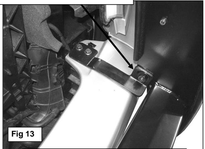
Titan & 04-07 Armada pictured without grille for photo purposes only. Reinstall grille before attaching Grille Guard
