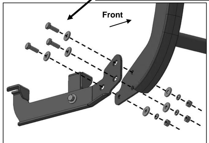
**(Fig 16) Attach Grille Guard to Frame Brackets**
