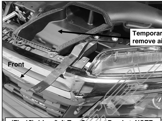
**(Fig 15) driver/left Top Support Bracket. NOTE:
