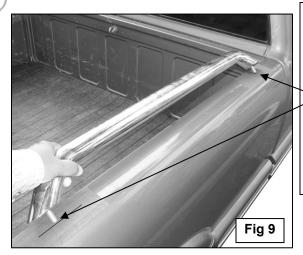
Hold the front of the Bed Rail in position with the point on the Stud in the center of the front drill location. Line up the rear Stud with the line scribed in Step 4, Fig 7. Use the point on the Stud to leave a small mark on the tape. Remove the Bed Rail and clearly mark the drill location. Drill a 7/16" hole through the front location. Insert the Bed Rail and check rear measurement before drilling through rear location
