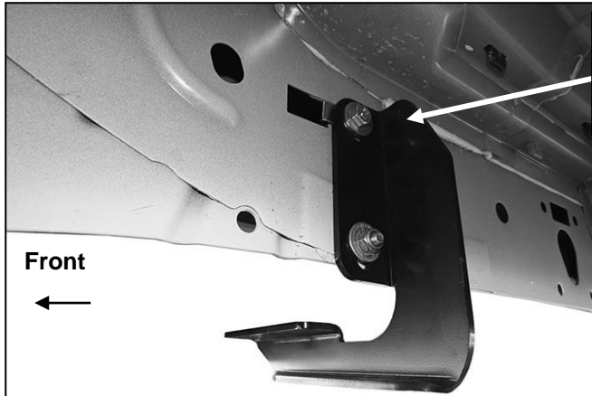
(Fig 3) Passenger/right front Bracket installed
