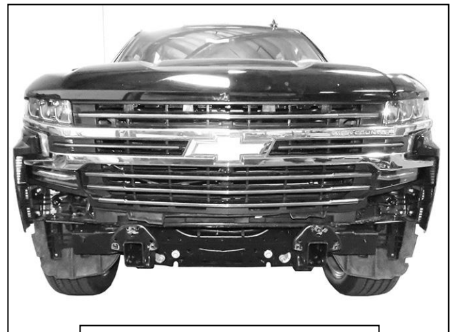
(Fig 6) Reinstall grille and cover
