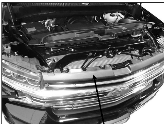
(Fig 1) Remove cover and screws attaching grille
