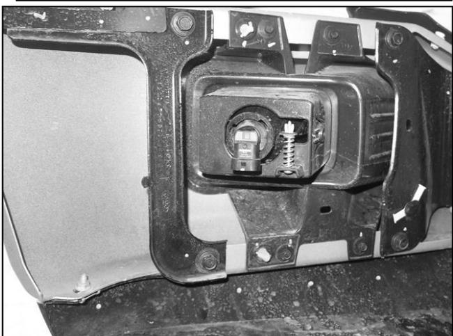
(Fig 11) Remove fog light assembly from bumper
