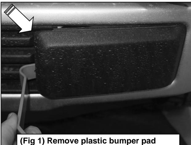
(Fig 1) Remove plastic bumper pad from bumper (Driver/left side Pictured)
