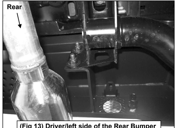
(Fig 13) Driver/left side of the Rear Bumper attached to the factory hitch
