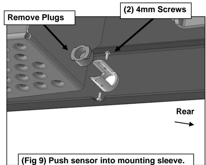
**(Fig 9) Push sensor into mounting sleeve. Use 4mm Screws to lock sensor in place.**
