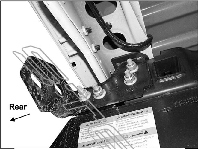
(Fig 3) Remove bumper bracket from frame
