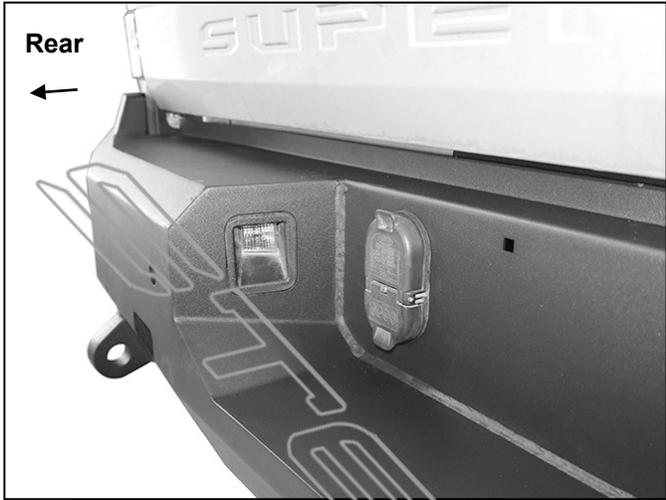
(Fig 11) Install wiring harness, trailer plug, license plate lights and spare tire access lock before installing Bumper
