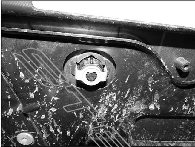
(Fig 7) Remove sensors, wire harness, license plate lights, trailer plug and spare tire access lock (pictured) if equipped
